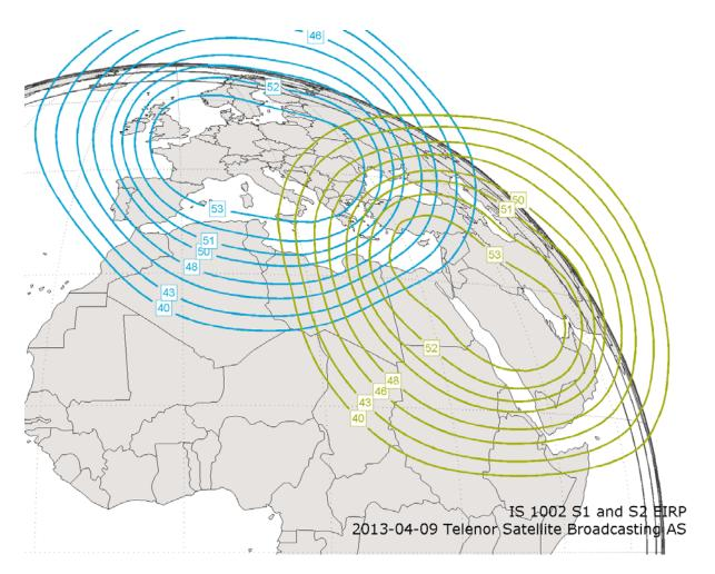
Cross pol test required when the uplink station is situated in the crossover region of spot 1 and spot 2 as above.
